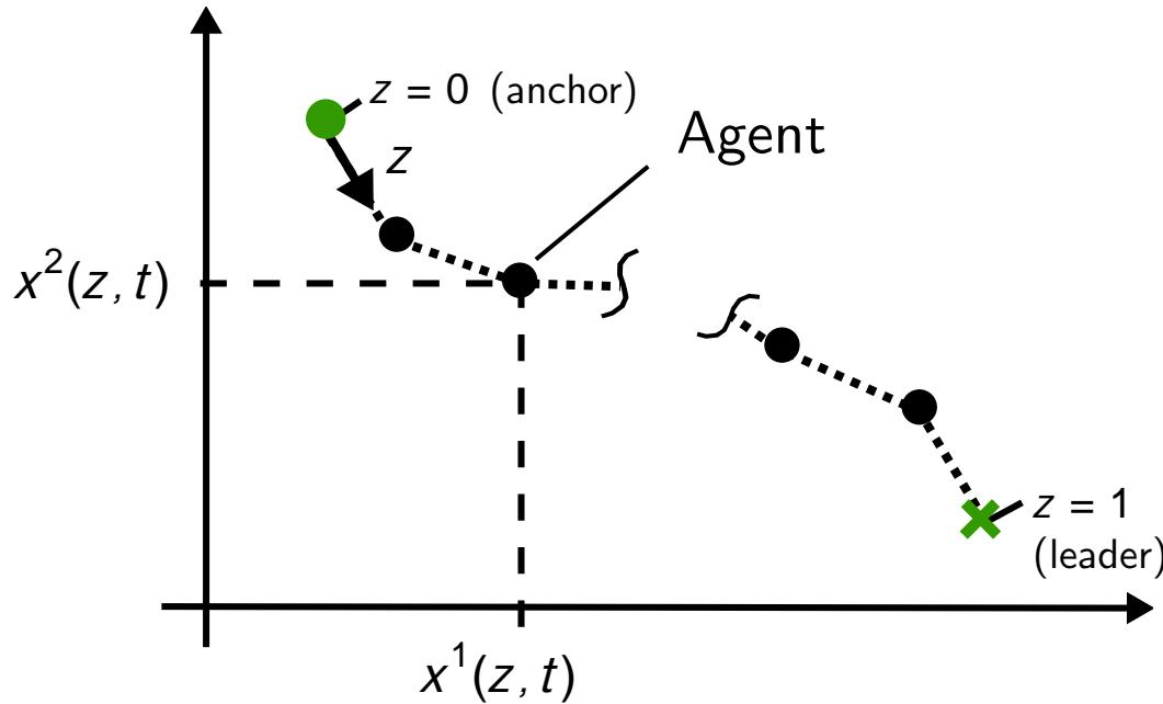
$$\begin{aligned} \text{PDE: } \partial_t x^i &= a^i \partial_z^2 x^i - b^i x^i \partial_z x^i + c^i(t) x^i \\ \text{BCs: } x^i(0, t) &= u_a^i(t), \quad x^i(1, t) = u_l^i(t) \\ \text{ICs: } x^i(z, 0) &= x_0^i(z) = 0, \quad i = 1, 2 \end{aligned}$$
