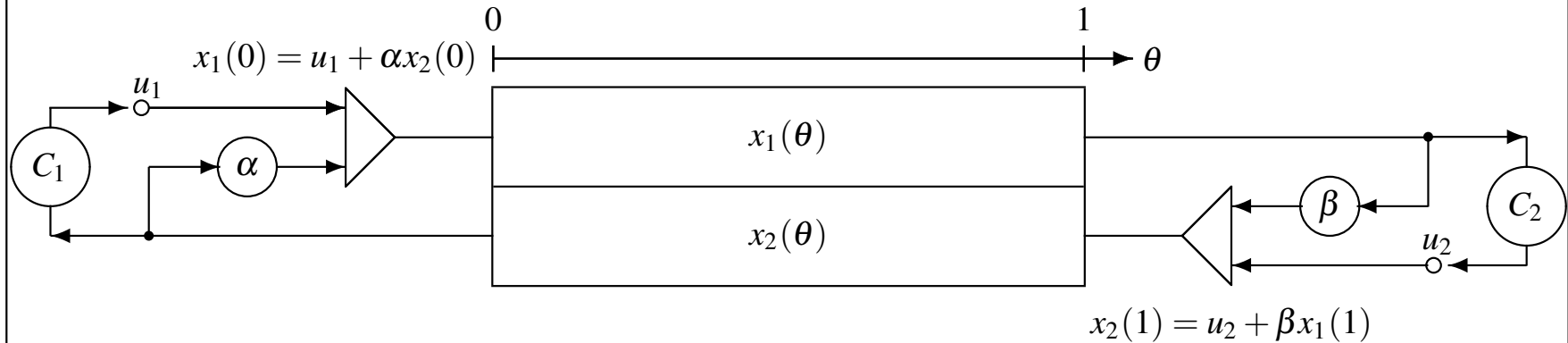
Figure 6.1: Open/closed-loop control system for the Chapelon–Xu example; C_1 := \frac{n}{m} - \alpha , C_2 := \frac{p}{q} - \beta .
